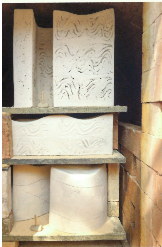
Aarti Vir's 0.6 m 3 down-draught woodfire saltglaze kiln packed and ready for firing at her studio in Hyderabad, India. It has a single firebox beneath the chamber and firings to 1300°C take 24 hours.
